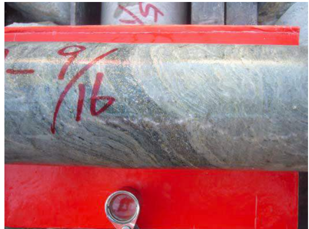
Photo 6-2 Target 2, Hole ZK1701, fine grained pyrite, sphalerite and galena bands occur along foliation
