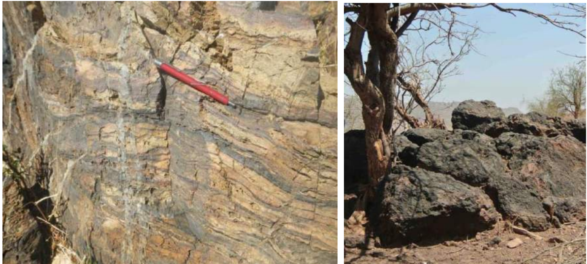
Photo 7-3 a) Banded iron formation with magnetite and chert Photo 7-3 b) massive iron oxide gossan at Adi Ekele zone
